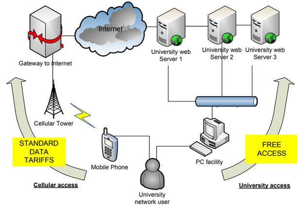
Fig. 1. Standard layout of cellular and Ethernet access on a campus
