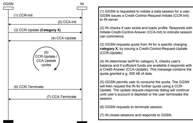
Fig. 2. Prepaid GPRS charging implemented using Diameter Credit Control Application (DCCA) protocol
