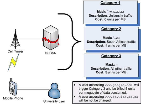
Fig. 3. eGGSN metering allows different tariffs dependent on URL
