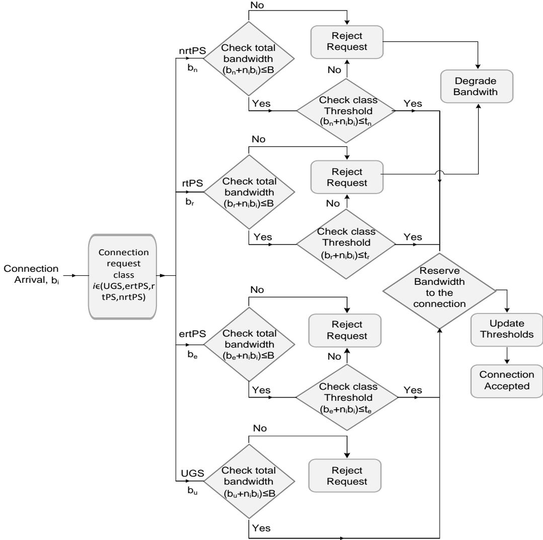
Figure 3: Connection Admission Control Operation Flow Chat
