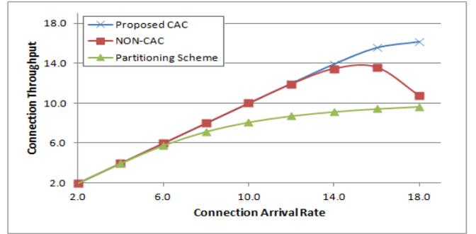
**Figure 4: Connection Throughput of the Proposed Scheme and other CAC Schemes**
