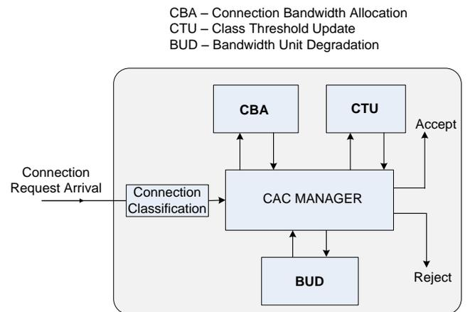
Figure 2: Connection Admission Control Framework
