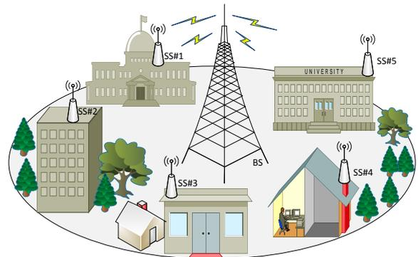
Figure 1: The PMP Operation Mode
